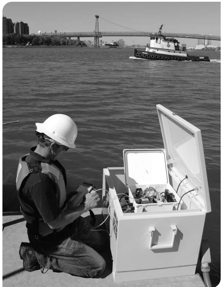
An example of a NEMA enclosure where the DCP Signal Output Adapter is wired.
