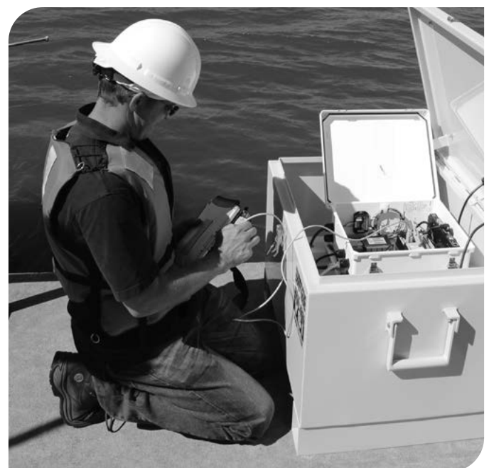
An example of a NEMA enclosure where PLC + Modbus adapter are wired.
